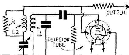
Fig. 1.—Experimenters should find this regeneration circuit of particular interest. It is suitable for use in all types of straight receivers.
