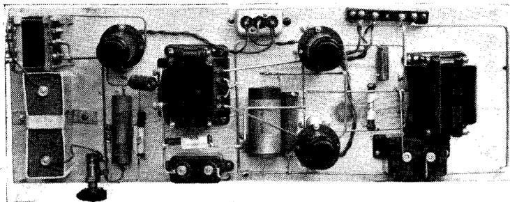
*All connections are made with heavy gauge wire, for with portable work nothing must come loose. The layout of the components can be seen from this illustration.*
