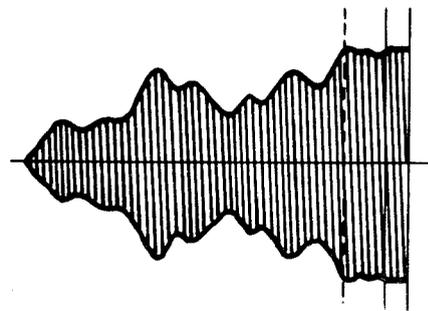
Fig. 2.—If a black part occurs in the picture before the pulse it causes the synchronising to be irregular.
