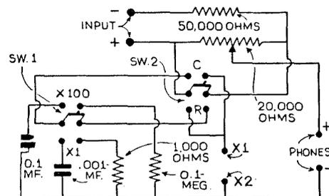
Fig. 2.—The capacity bridge.
