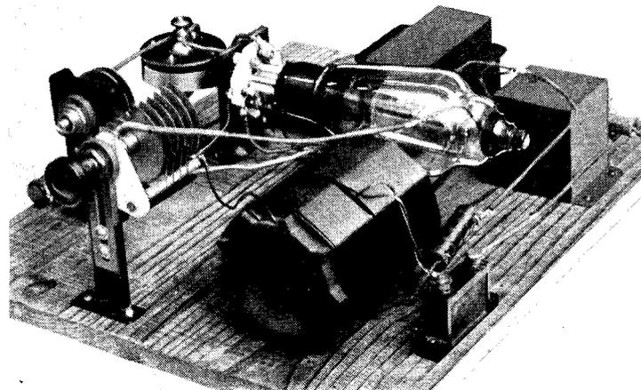
*The coil shown in this illustration covers the 160 metre band, but it can be modified for use on 80, 40 or 20 metres.*
