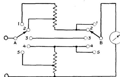
5. The switching arrangements in Figs. 3b and 4b can be used to form a combined voltmeter and milliammeter in this way.
