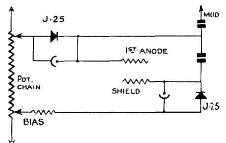
Fig. 2.—Double Modulation circuit employing metal rectifiers
