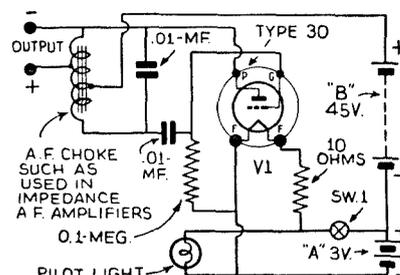
Fig. 3.—The low-frequency oscillator.
