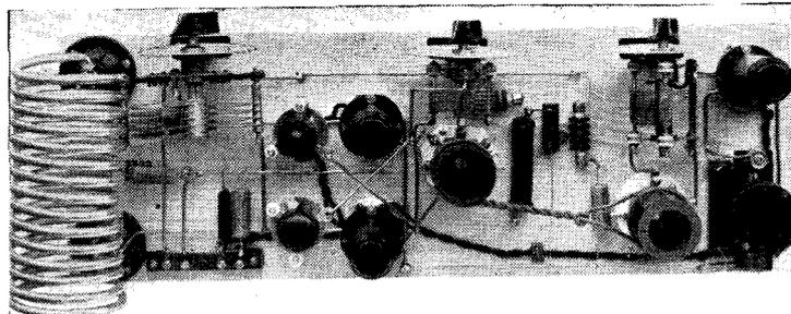
A good idea of the layout of the components can be obtained from this plan view. A crystal stage is on the extreme right, which is link coupled to a pair of valves to the left.
