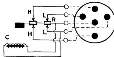
The Bulgin H.T. vibrator is made up internally in this way. The multi-contacts explain the need for so many buffer condensers.
