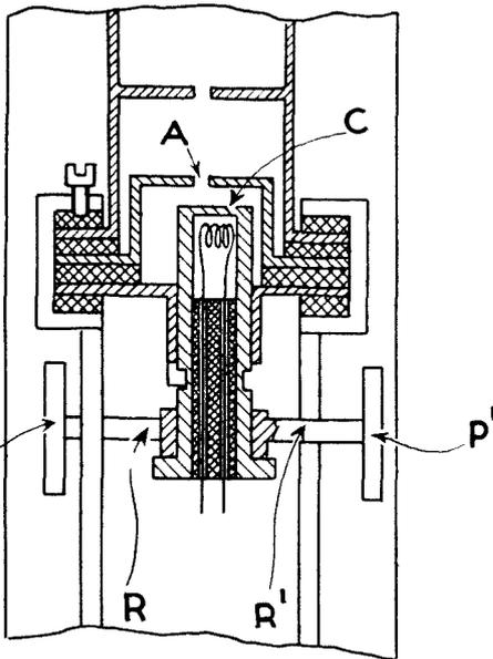
*Construction of cathode-ray tube with rotatable cathode in order to change the operative part of the cathode surface. Patent No. 462,243.*
