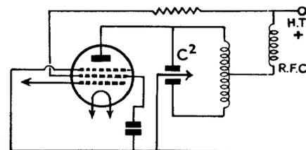
Fig. 3. Greater radio frequency output for a given input can be obtained from a pentode valve in this type of circuit.
