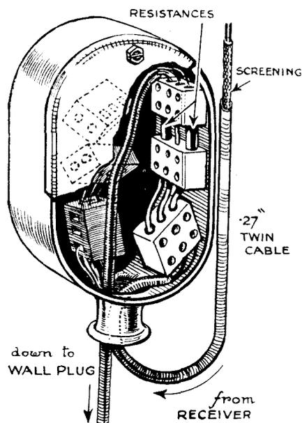
*A junction box is provided in each flat which contains the connectors and resistances for television and radio relay.*
