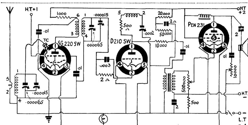
The numbers on the coils agree with the numbers that can be found on the base of the Eddystone coil holders. These should be strictly followed.
