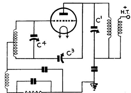
Fig. 7. A grid neutralised circuit of this kind is very effective, while the tuned circuit permits of easy coupling to the previous stage.
