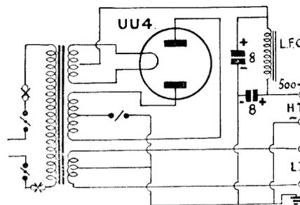
*A power pack of this kind is required for the transmitter. It gives a maximum of 500 volts at 120 M/a.*
