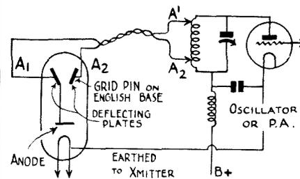
*This miniature cathode-ray tube can be connected very simply to a C.W. transmitter, and, as explained in the text, has numerous uses.*
