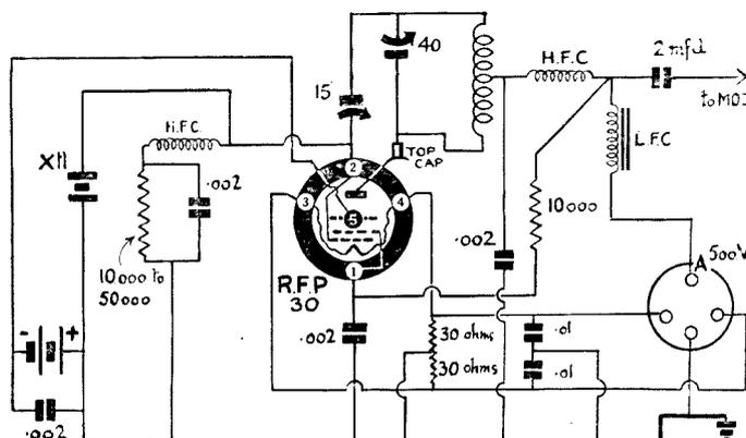
*This simple circuit includes all the components as well as the modulation choke. The voltage applied should be adjusted so that the maximum input is 10 watts.*
