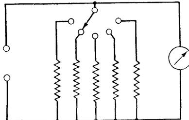
Fig. 2. If a milliammeter is shunted in this way it can cause considerable error.
