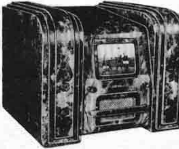
Above—The new Television Receiver made by an Italian company. The size of the image projected by the cathode-ray tube measures 8 by 10 inches, 240 lines, at 25 frames per second. Price, $640.00! Loudspeaker grill shown below image.
