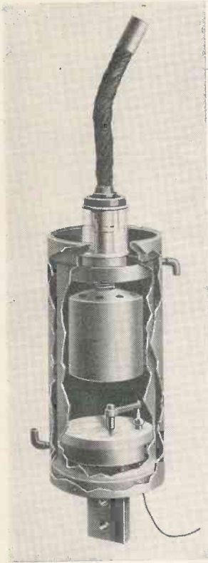
Fig. 3. Type BK24 Ignitron cut away to show general arrangement.
