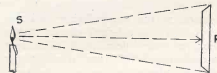
Fig. 1. Diagram showing how luminous intensity is determined.
